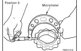
2. Measure the inner diameter of oil pump body with inside micrometer (Position 6) (Clearance) = (Inner diameter of oil pump body) - (Outer diameter of inner rotor)
